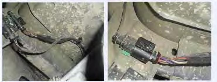
Connect to OE central lock cables (Violet and Brown) at gastank cap.
